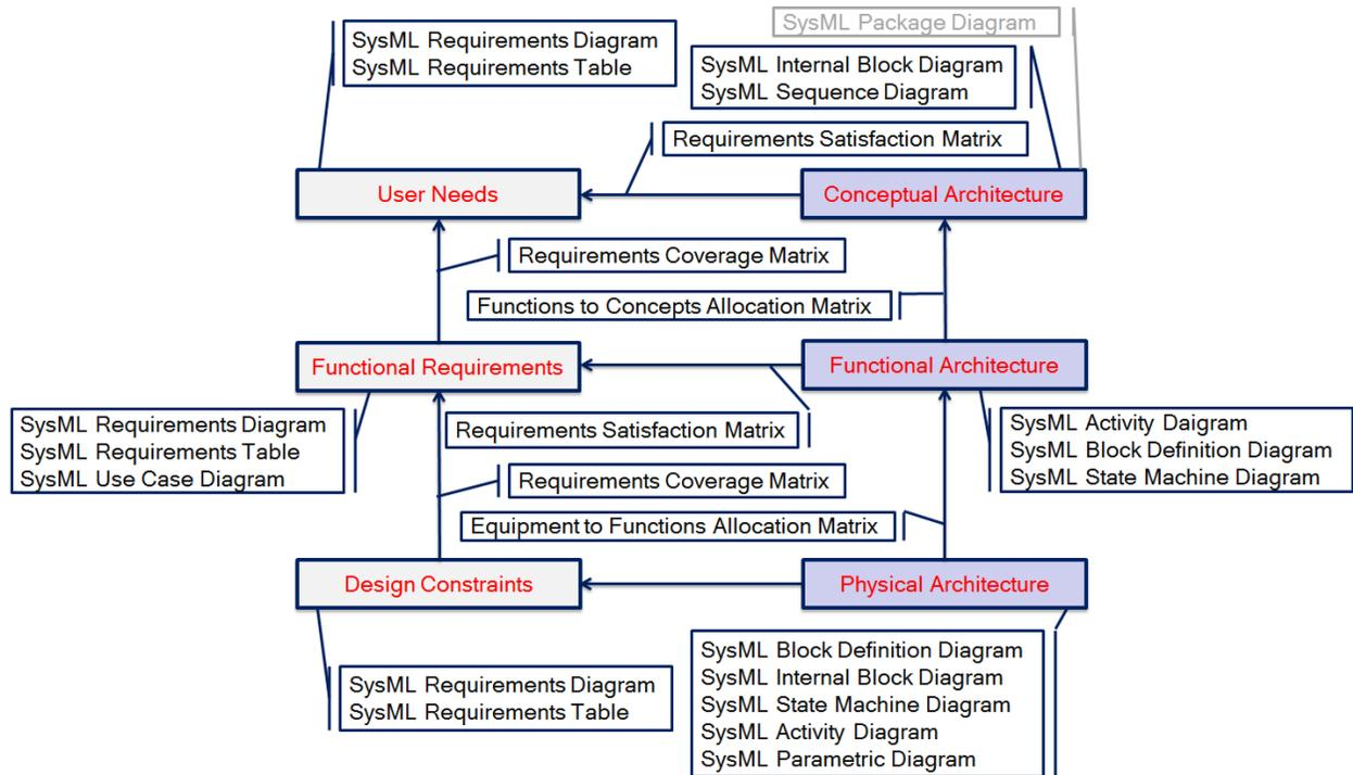
Figure 3 Architectural Models to SysML Diagrams Mapping
